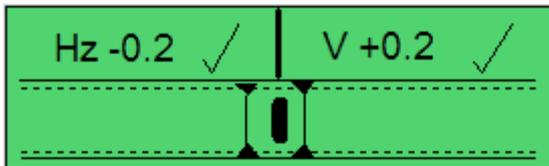
Once the supplies are in sync, the module initiates a breaker close signal placing the two supplies in parallel. If synchronism is broken or not achieved, the moving bar passes out of the synchronising window.
