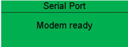
In case of communication failure between the modem and module, the modem is automatically reset and initialisation is attempted once more:
