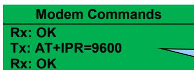
Shows the last command sent to the modem and the result of the command.
