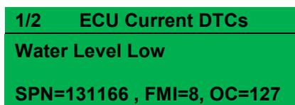
The DM1 DTC is interpreted by the module and is shown on the module's display as a text message. In addition to this, the manufacturer's DTC is shown below.
