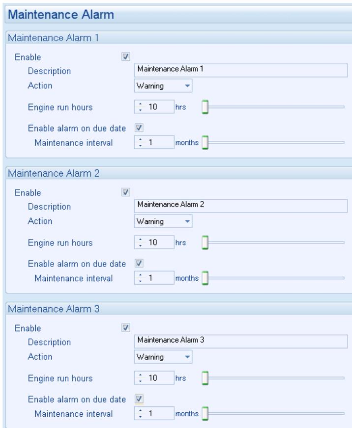
The screenshot displays three separate configuration panels for Maintenance Alarm 1, Maintenance Alarm 2, and Maintenance Alarm 3. Each panel contains the following settings:
