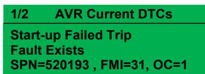
The DM1 DTC is interpreted by the module and is shown on the module's display as a text message. In addition to this, the manufacturer's DTC is shown below.
