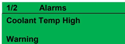
In the event of an alarm the LCD jumps to the alarms page, and scroll through all active alarms.
