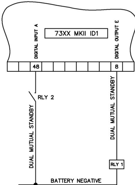
In case of set 1 failure, the output activates and energises the external relay RLY1 to call for the second set to start.
