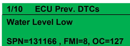
The DM2 DTC is interpreted by the module and is shown on the module's display as a text message. In addition to this, the manufacturer's DTC is shown below.
