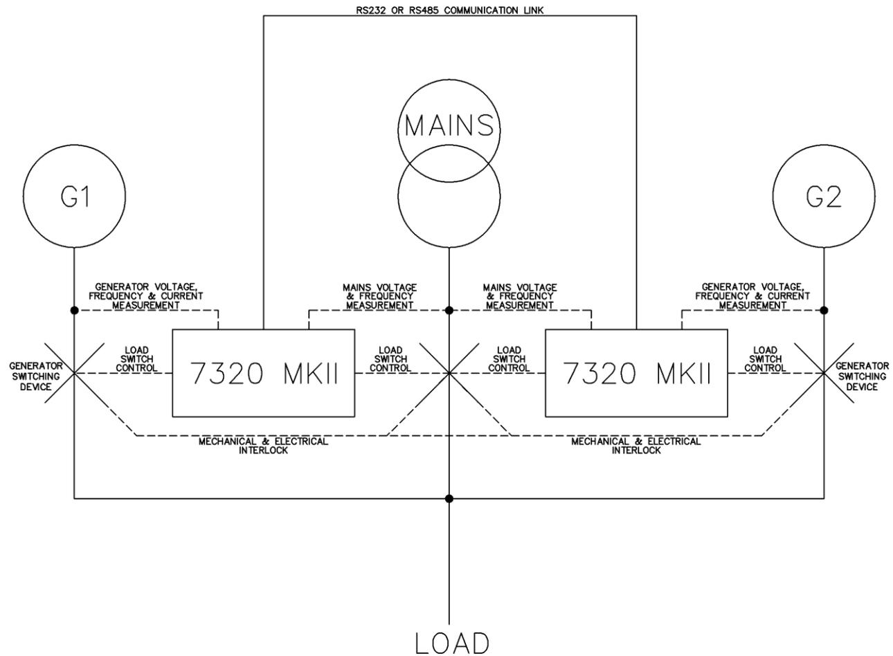
3.3.6.3 TWO DSE73XX MKII USING DIGITAL INPUTS AND OUTPUTS
