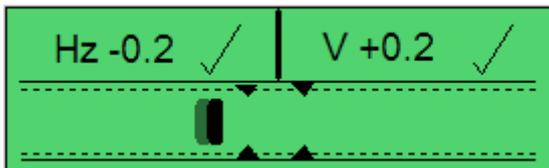
If the DSE module is configured to do so, it actively controls the synchronising using a CANbus engine and CANbus AVR. The module first matches the frequency and voltage and when they are within acceptable limits, the phase matching begins as indicated by the moving bar which shows the phase difference between the two supplies. The engine speed is automatically adjusted, altering the phase, until the moving bar enters the centre of the scope.
