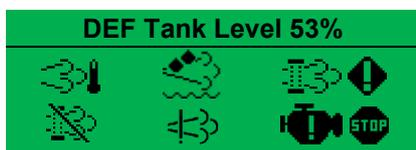
For further information about the default icons, refer to *Engine* section elsewhere in this manual. Depending upon module configuration, the icons displayed and their functions may differ from the default. An example of icon configuration is shown:
