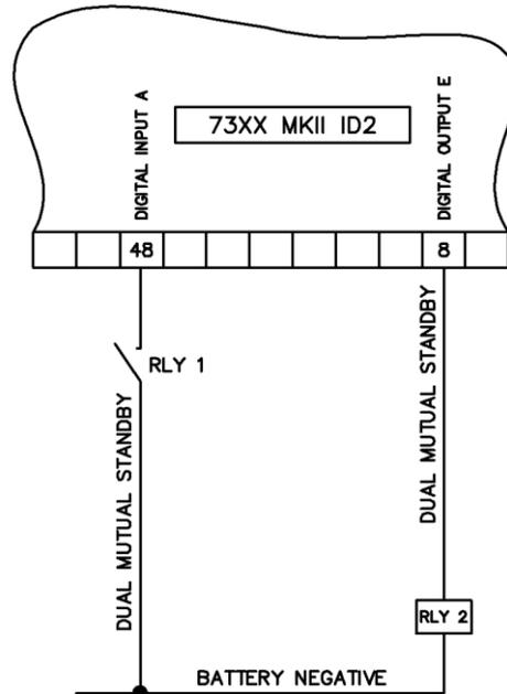
RLY1 contact closes a battery negative signal onto the input, instructing the set to start.
