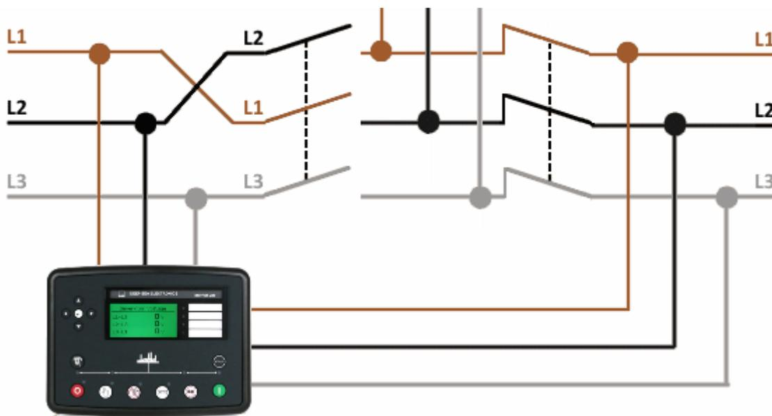
This is tested by starting the generator with the DSE module and ensuring the generator switchgear is left open (activate an input configured for *Generator Load Inhibit*). Then the load bus is to be made live, this is achieved by ensuring the mains switchgear is closed. Across the switchgear, connect a voltage meter to measure the AC voltage when the DSE module shows the two supplies in sync.
