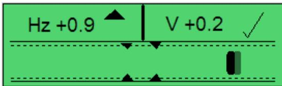
Initially the synchroscope display shows the difference between the bus and generator supplies. Here the display is showing a frequency mismatch of +0.9 Hz and a voltage mismatch of +0.2 V. The genset frequency is too high (indicated by the arrow) and must be reduced. The voltage is high, but is within the check sync limits set for synchronising (indicated by the tick). In most cases, the DSE module then waits for the frequency, voltage and phase to drift into synchronism.
