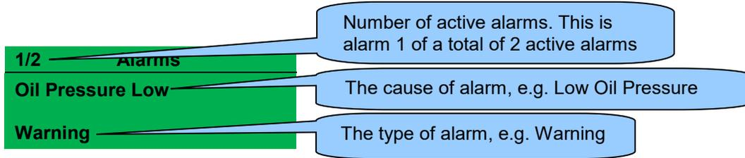
The LCD displays multiple alarms such as "*Coolant Temperature High*", "*Emergency Stop*" and "*Low Coolant Warning*". These automatically scroll in the order that they occurred or press the
