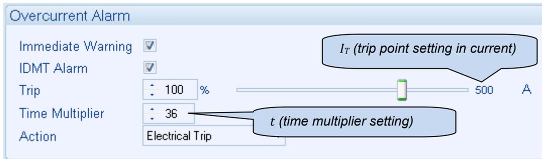
These settings provide for normal running of the generator up to 100% full load. If full load is surpassed, the *Immediate Warning* alarm is triggered and the set continues to run.
