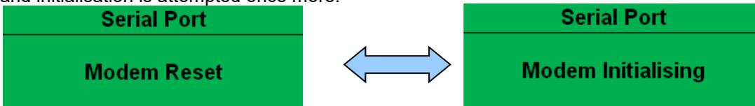
In the case of a module that is unable to communicate with the modem, the display continuously cycles between 'Modem Reset' and 'Modem Initialising' as the module resets the modem and attempts to communicate with it again, this continues until correct communication is established with the modem. In this instance, check connections and verify the modem operation.
