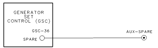
Illustration 52 System Schematic For Spare Output When used as a high/low logic circuit.
