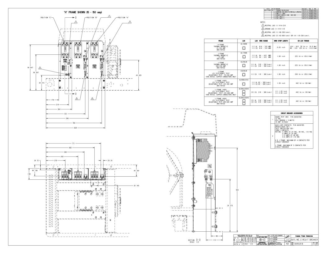
FIGURE 64. CIRCUIT BREAKER OUTLINE (SHEET 1 OF 3)
