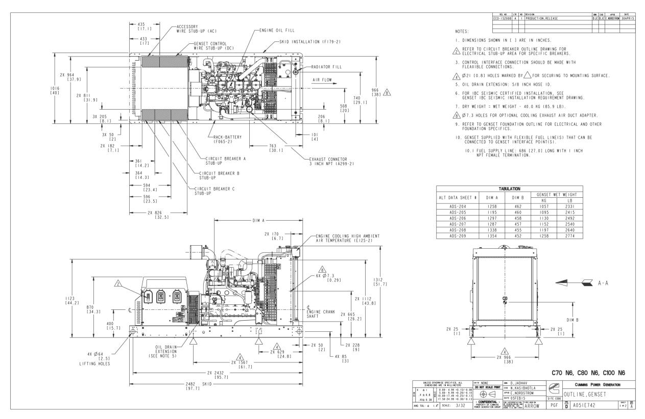
FIGURE 28. GENERATOR SET OUTLINE, 70-100 KW (SHEET 1 OF 2)
