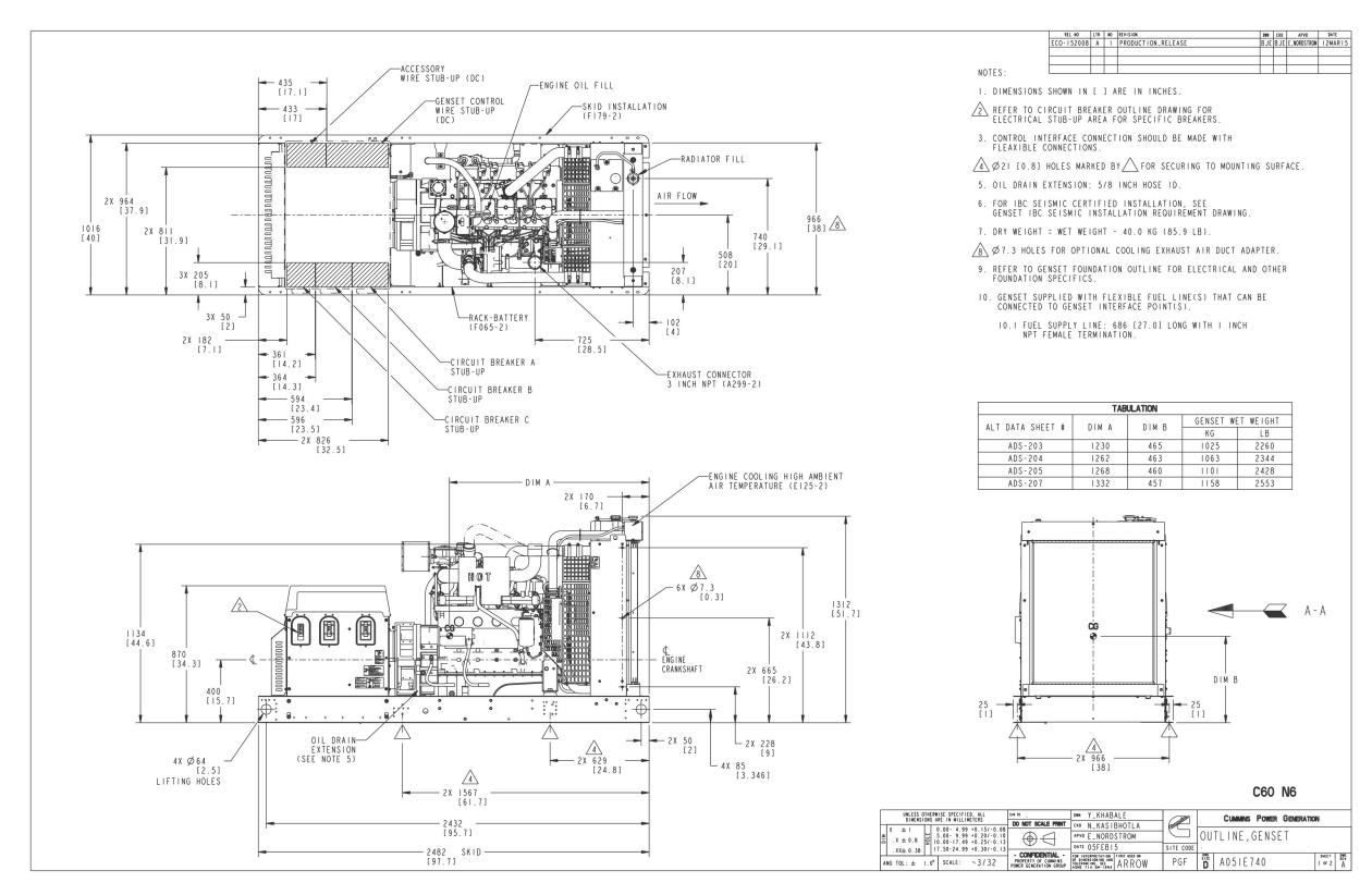
FIGURE 26. GENERATOR SET OUTLINE, 60 KW (SHEET 1 OF 2)
