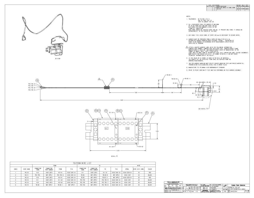
FIGURE 71. RELAY HARNESS (SHEET 1 OF 1)
