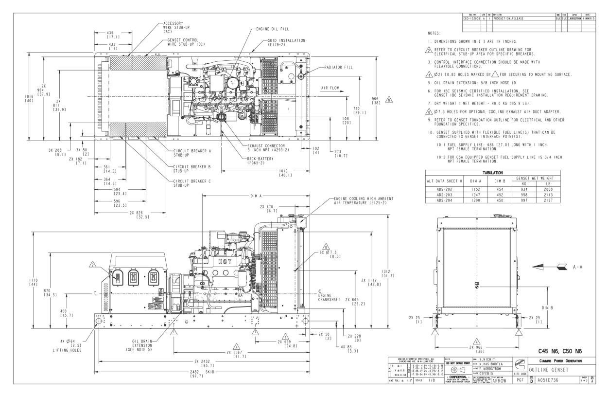
FIGURE 24. GENERATOR SET OUTLINE, 45-50 KW (SHEET 1 OF 2)
