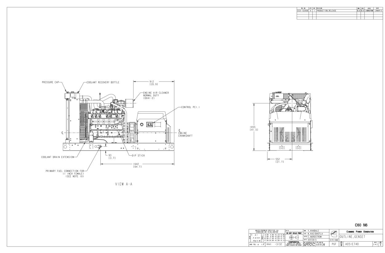
FIGURE 27. GENERATOR SET OUTLINE, 60 KW (SHEET 2 OF 2)
