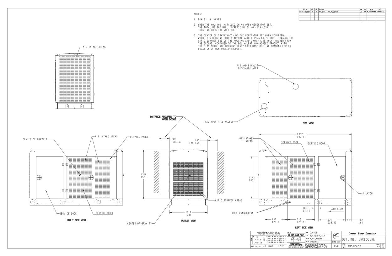
FIGURE 33. ENCLOSURE OUTLINE, WEATHER (SHEET 1 OF 1)
