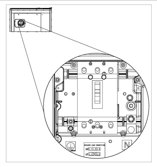
FIGURE 7. CIRCUIT BREAKER AC LOAD CONNECTIONS LOCATION (SYMBOLS SHOWN AT BOTTOM)
