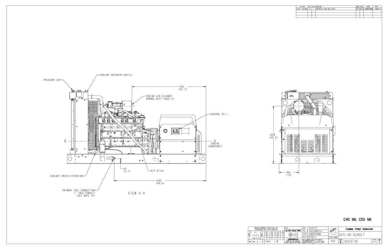
FIGURE 25. GENERATOR SET OUTLINE, 45-50 KW (SHEET 2 OF 2)
