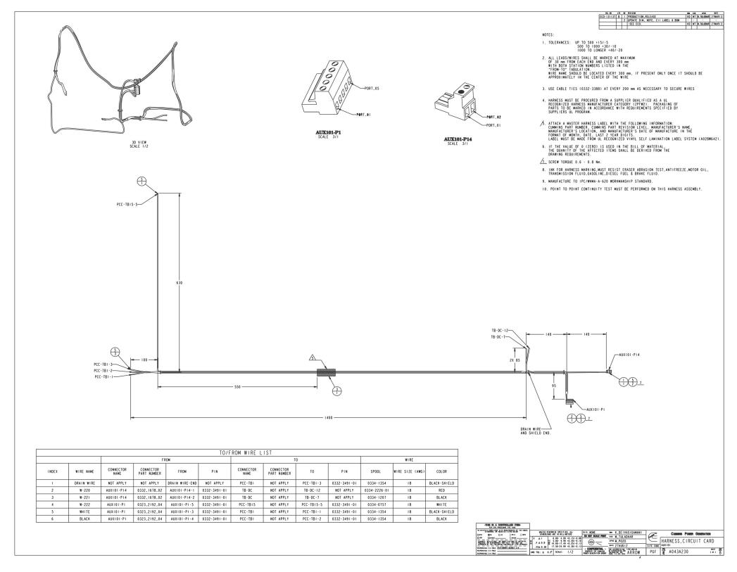
FIGURE 70. CIRCUIT CARD HARNESS (SHEET 1 OF 1)
