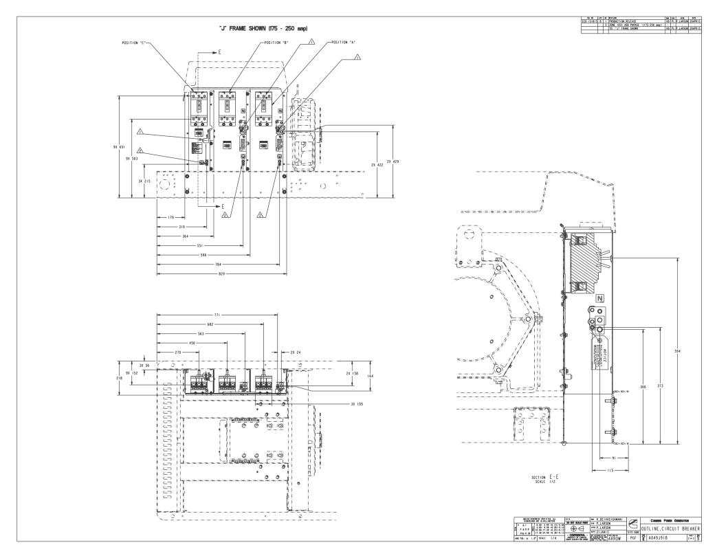
FIGURE 65. CIRCUIT BREAKER OUTLINE (SHEET 2 OF 3)
