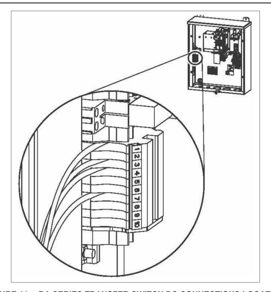
FIGURE 11. RA SERIES TRANSFER SWITCH DC CONNECTIONS LOCATION
