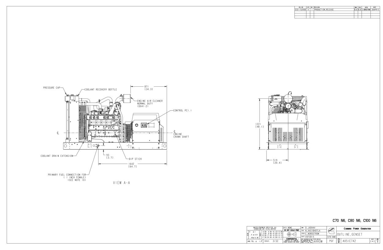
FIGURE 29. GENERATOR SET OUTLINE, 70-100 KW (SHEET 2 OF 2)
