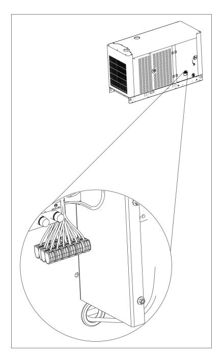
FIGURE 10. DC CUSTOMER CONNECTIONS
