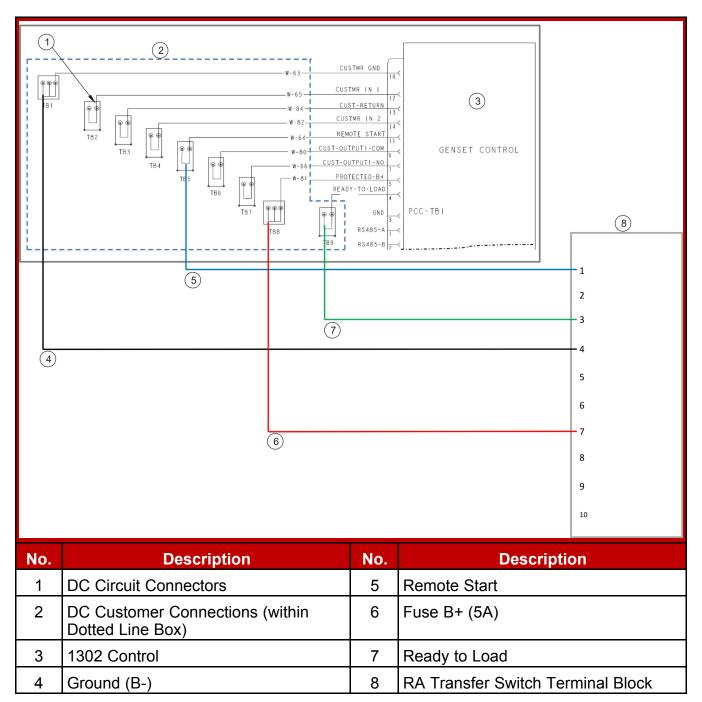
FIGURE 12. GENERATOR SET TO RA TRANSFER SWITCH DC CUSTOMER CONNECTIONS
