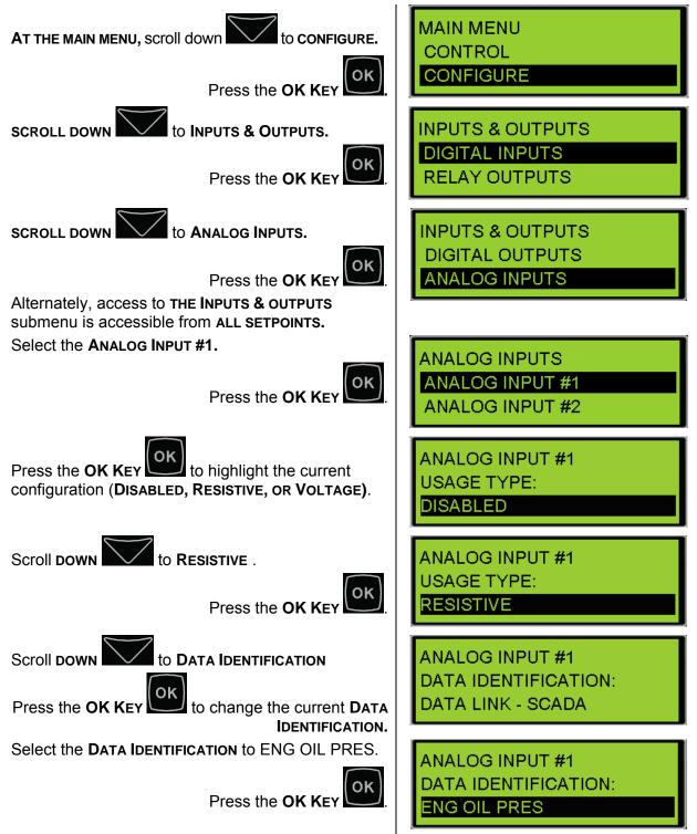
to configure the remaining setpoints for Analog Input #1:
