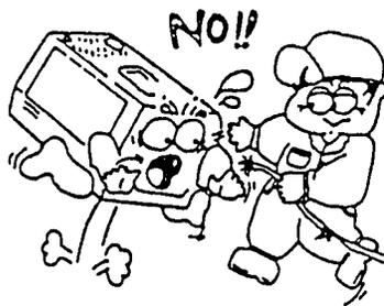
■ **Never** use damaged or worn cables when connecting power tools or equipment to the generator. Make sure power connecting cables are securely connected to the generator's output terminals, insufficient tightening of the terminal connections may cause damage to the generator and electrical shock.
