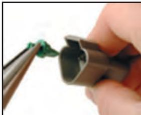
1. Remove wedgelock using needle-nose pliers or a hook shaped wire. Pull wedge straight out.
