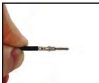
1. Grasp crimped contact approximately (25.2 mm) one inch behind the contact barrel.
