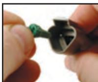
4. Once all contacts are in place, insert wedgelock with arrow pointing toward exterior locking mechanism. The wedgelock will snap into place. Rectangular wedges are not oriented. They may go in either way. **NOTE:** The receptacle is shown –use the same procedure for plug.
