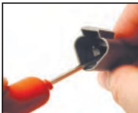
2. To remove the contacts, gently pull wire backwards, while at the same time releasing the locking finger by moving it away from the contact with a screwdriver.
