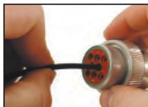
3. Push contact straight into connector grommet until a positive stop is felt. A slight tug will confirm that the contact is properly locked in place.
