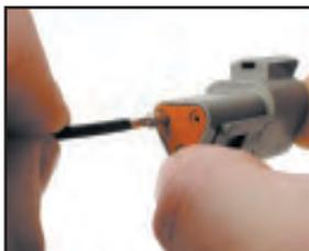
3. Hold the rear seal in place, as removing the contact may displace the seal.
