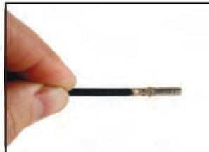
1. Grasp contact approximately (25.4 mm) one inch behind the contact crimp barrel.
