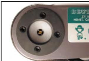
4. Insert contact with barrel up. Turn adjusting screw counter-clockwise until contact is flush with indenter cover. Tighten locknut.
