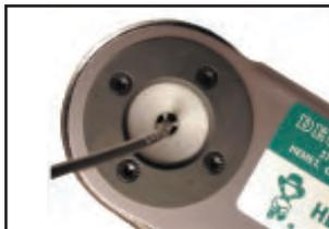
5. Insert wire into contact. Contact must be centered between indicators. Close handles until crimp cycle is completed.
