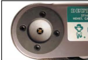
4. Insert contact with barrel up. Turn adjusting screw counter-clockwise until contact is flush with indenter cover. Tighten locknut.
