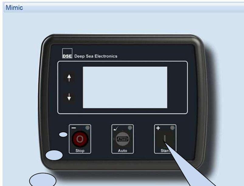
Click the mimic buttons to control the module remotely
